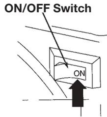
**⚠ CAUTION** You **MUST** unplug any load from the generator before starting to prevent permanent damage to any appliances.
