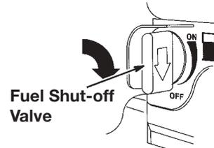
**NOTE:** When engine is transported, close fuel shut-off valve to prevent leakage.
