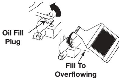
**NOTE:** When adding oil to the engine crankcase, use a high quality detergent oil classified "For Service SF,SG,SH" rated SAE 30 weight. Use no special additives. Select the oil's viscosity grade according to your expected operating temperatures.
