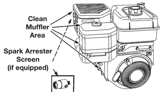
Remove spark arrestor screen for cleaning and inspection every 50 hours or every season. Replace if damaged.
