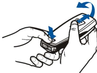
2. Lift the battery out of the phone, the bottom part first.
