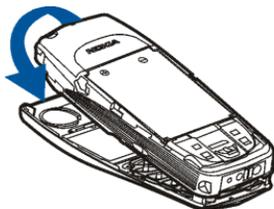
5. To replace the back cover of the phone, direct it towards the locking catches on the front cover and slide the back cover until it locks into place. See [Installing the SIM card and the battery](#) on page 18.
