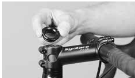
Retire a tampa terminal
