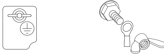
Figure 3-2 Frame Ground Connection
