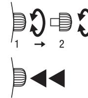
The crown also acts as a pusher to activate different functions such as the arming and disarming of the alarm, and to operate the three chronograph functions: starting, stopping and resetting to zero.
