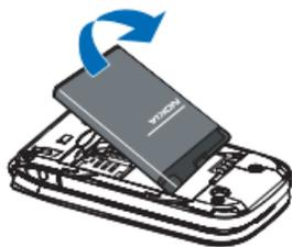
3. Position the battery so the gold-coloured contacts match up with those on the phone, and insert the battery into the battery slot.
