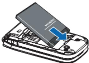
4. Push down on the other end of the battery to snap the battery into place.
