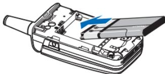
2. Push down on the other end of the battery to snap the battery into place.
