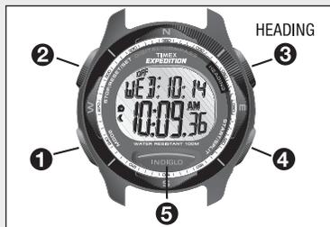
Press **1** to cycle through time/date, chronograph, countdown timer, alarm. Compass function available in all modes except alarm by pressing **3** (HEADING).
