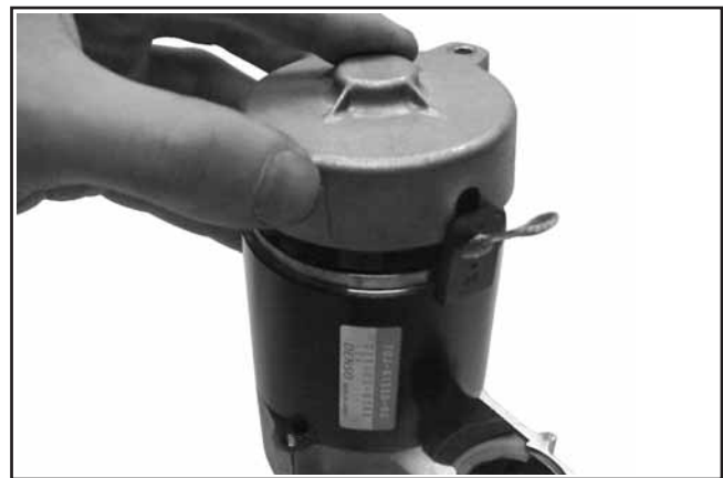
Figura 8-26. Instalar a Tampa Terminal.
