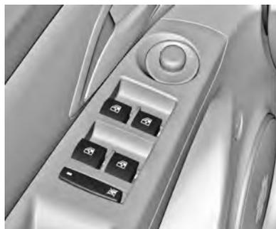
Pressione o interruptor
