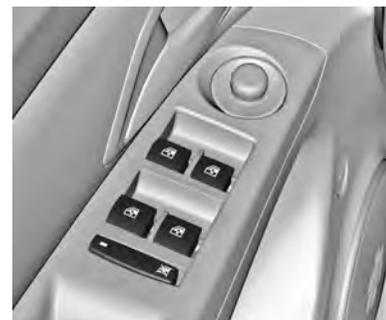
Pressione o interruptor
