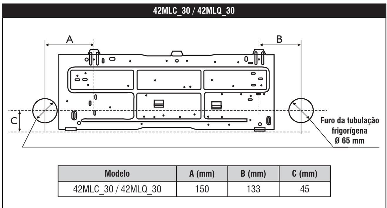
FIG. 20 - PLACAS DE MONTAGEM
