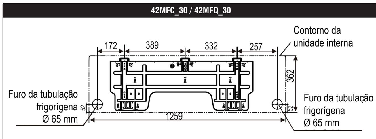
FIG. 20 - PLACAS DE MONTAGEM
