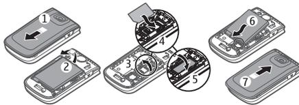
1. Press and slide the back cover toward the bottom of the device to remove the cover (1).
