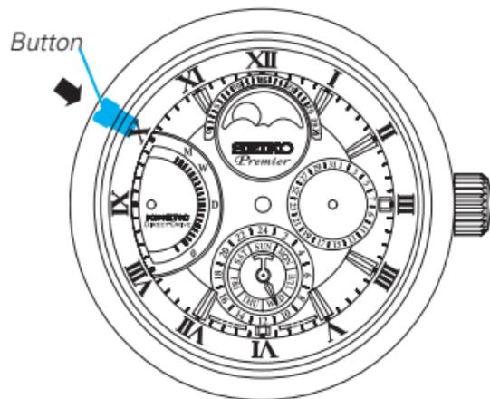
1. Press the button using an object with a long tapered tip such as a ballpoint pen.
