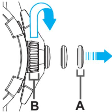
To pull out the crown, pull out the **A portion** (crown).
