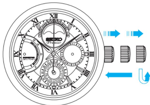
1. Pull out the crown to second click when the second hand is at the 12 o'clock position.
