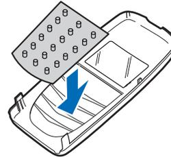
3. Press the front cover and keymat against the phone, and snap the front cover into place.
