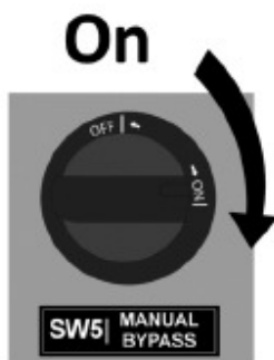
Figura 41 - Ligando o interruptor de bypass manual (SW5)
