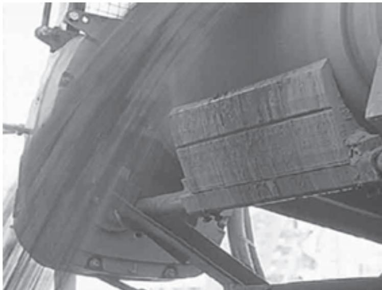
**Figura 44 – Raspadores *Martin Engineering***
