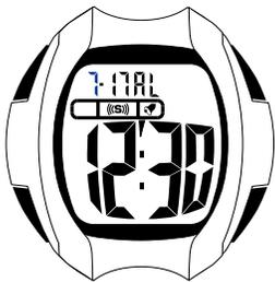
The vibration and sound alarms will operate together for 30 seconds, and can be stopped by pressing any key.
