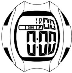
To use the timer in a count up state, press the ST/STP button to start from zero. Press the ST/STP button to stop. Press RESET button to reset to zero.
