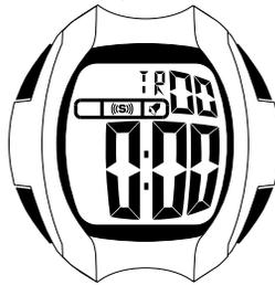
Press MODE button to change to the next item, setting sequence will be a cycle by seconds, minutes and hours. Press ST/STP button to adjust the flashing digits. Once desired time has been set press the EL/SET button to exit the Timer Setting Mode or press the ST/STP button to begin the countdown timer.
