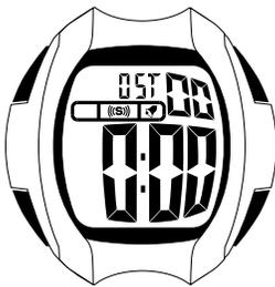
To measure elapsed time, press the ST/STP button to start the counter. Press the ST/STP button to stop the counter.
