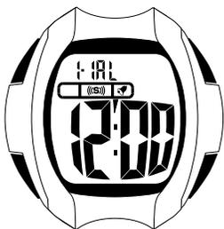
Press MODE button to change to the next item, setting sequence will be a cycle by minute, hour, month and date. Be sure that schedule alarm is off by deleting the month and date:
