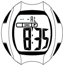
Press the ST/STP button to adjust the flashing digits. Once everything has been set press EL/SET button to exit the Alarm Setting Mode.
