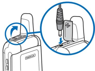
1. Plug the charger transformer into a standard ac outlet.
