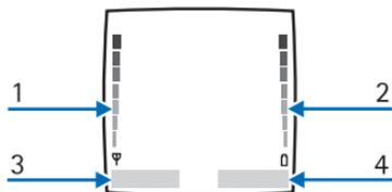
Signal strength (1)—A higher bar indicates a stronger network signal.
