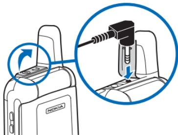
1. Plug the headset connector into the connector at the top end of your phone.
