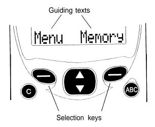
For example, the **Menu** selection key (key under the text Menu) gains access to the menu functions and the **Memory** selection key (key under the text Memory) to the memory functions.
