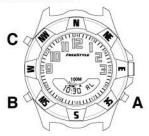
From normal time mode, press mode button C once to enter alarm mode. "ALM" will flash on upper left side of display. To set alarm, press and hold set button **B** for about three seconds; hour digits will flash.Press start/stop button A to advance hour digits; hold for rapid advance. Press set button B; minutes digits will flash. Press start/stop button A to advance minutes digits; hold for rapid advance. Press MODE button C to complete alarm setting at any time.
