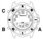
Press start/stop button A to reset seconds digits to "00". If seconds are greater than 30, one minute will be added to the minutes
