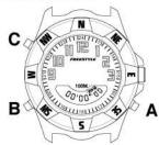
From date mode, press mode button C three times to enter chronograph mode. "STP.W" will flash on upper right side of display. Press start/stop button A to start (or stop) the chronograph counting.
