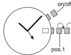
If your watch has an alarm function you can set the alarm by pulling out the 3 o'clock crown to position 1 and turning it in a clockwise direction. The shortest hand is usually the alarm hand. When the hand is set to the desired alarm time pull out the 2 o'clock crown to turn the alarm on. Alarm sounds for 15 seconds and is repeated for around 3 minutes. To turn alarm sounds off, push the 2 o'clock crown button fully in.
