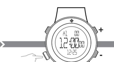
Press button S3 to advance through hour, minute, month, day, T1/T2, chime, adding or subtracting using buttons S1 or S2.
