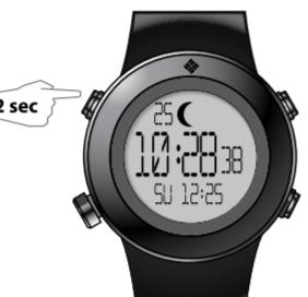
Press and hold button S4 for 2 seconds (the second digit will start flashing)
