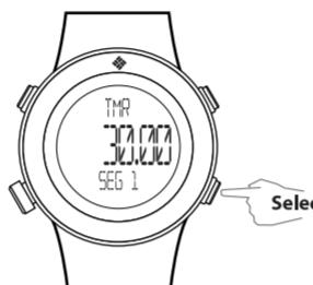
Press S3 to set seconds, minutes, hours, then segments. Press S1 and S2 for plus/minus.
