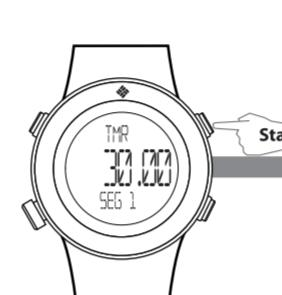
Press S2 to start countdown timer. Timer will switch automatically to other segment timer.
