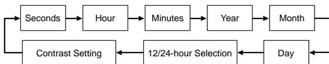
2. While a setting is flashing, use (E) (+) and (B) (-) to change it.
