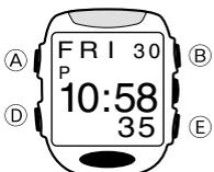
1. In the Timekeeping Mode, hold down (A) for about one second until the seconds digits start to flash on the display. This indicates the setting screen.
