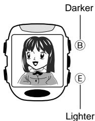
When composing an image on the display, use **B** (darker) and **E** (lighter) to adjust its brightness.
