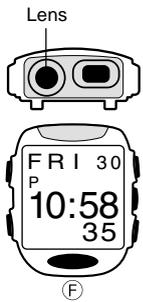
Use the Camera Mode to record images. The lens for image recording is located on the top edge of the watch.
