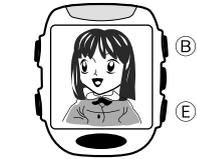
1. In the VISUAL DATABANK Mode, use **E** (+) and **B** (-) to display the image to which you want to attach text.
