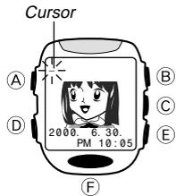
3. Press **F** to display the text input screen.
