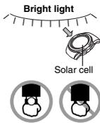
The electricity generated by the solar cell of the watch is stored by a built-in battery. Leaving or using the watch where it is not exposed to light causes the battery to run down. Make sure the watch is exposed to light as much as possible.
