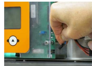
Retire o conector do terminal do Painel de Controle TEMP PROBE.
