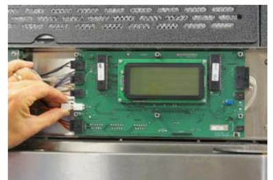
Retire todas as conexões do terminal do painel de controle principal.
