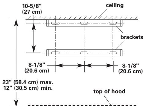
**Make sure that the screws are securely fastened to the wall.**
