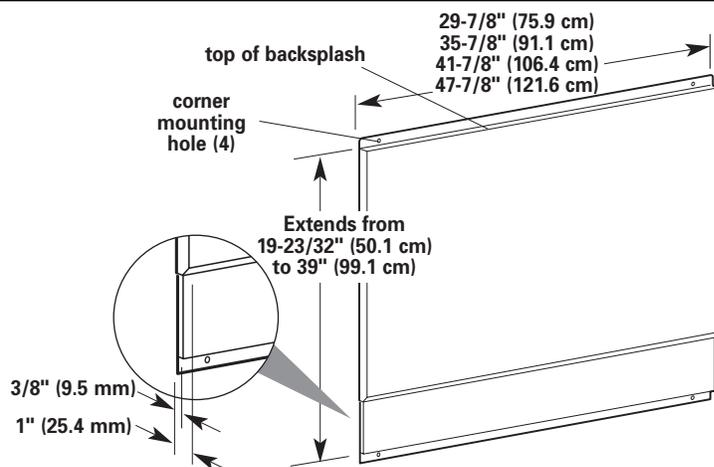
of the hood. Note: The minimum height of the hood above the cooktop, as shown on Page 3, is 30" (76.2 cm). The backsplash can be extended from 19-23/32" (50.1 cm) to 39" (99.1 cm). Note: As the 30" (76.2 cm) installation height **increases**, the hood's capture area **decreases**.
