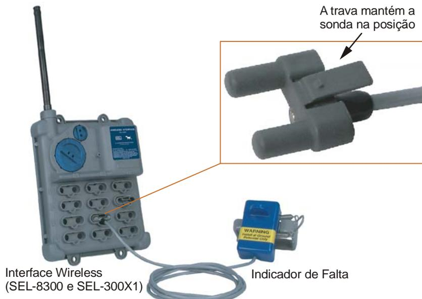
Figura 6 Insira as sondas magnéticas na Interface Wireless
