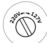
DETALHE DA CHAVE SELETORA DE VOLTAGEM
