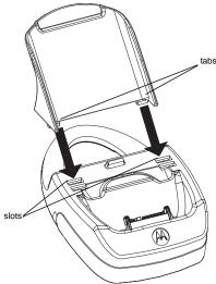
2 Press the phone support downward on to the base of the cradle, until it cannot easily be removed.
