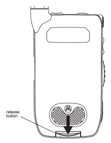
3 Allow the battery door to pop up, slide it forward, and remove it from the back of your Smartphone.
