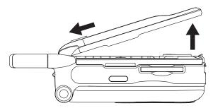
3 Insert the top of the battery into the battery area. Press the bottom of the battery to secure it.
