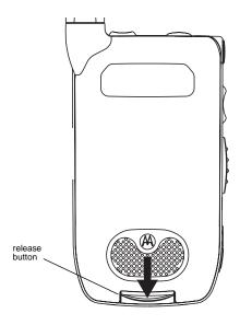
**3** Allow the battery door to pop up, slide it forward, and remove it from the back of your Smartphone.
