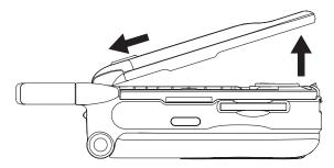
4 Remove the battery by pushing it toward the antenna and lifting it out.
