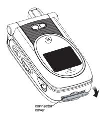
2 With the Smartphone's display facing up, insert the serial data cable's connector into the accessory connector, until you hear a click.
