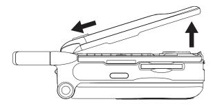
Your SIM (Subscriber Identity Module) card is a small piece of plastic located in the SIM card holder in the back of your Smartphone, underneath the battery.
