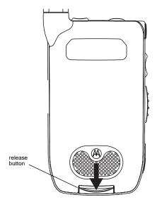
**2** Allow the battery door to pop up, slide it forward, and remove it from the back of your Smartphone.
