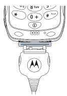
**Tip:** To remove the charger from the accessory connector: Press the buttons on the sides of the plug. Pull the plug straight out.
