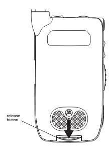
2 Allow the battery door to pop up, slide it forward, and remove it from the back of your Smartphone.
