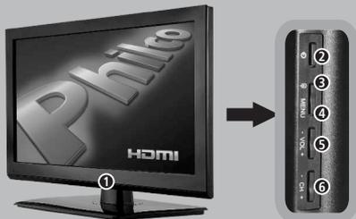
**1** SENSOR DO CONTROLE REMOTO E LED INDICADOR DO STANDBY.
