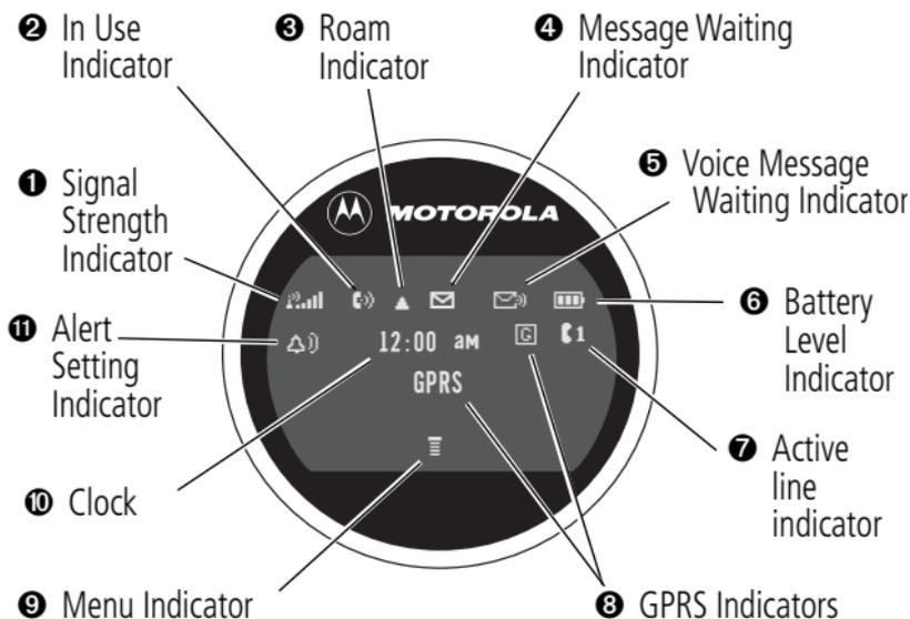
**1 Signal Strength Indicator** Shows the strength of your phone's connection with the network.
