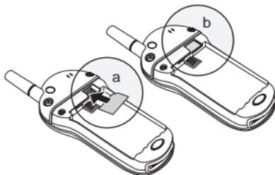
When the SIM card is properly positioned, the battery compartment terminals are visible.
