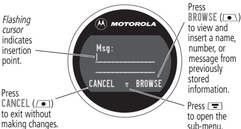
When you enter text, the flashing cursor changes to a *block cursor*, and the soft key functions change:00
