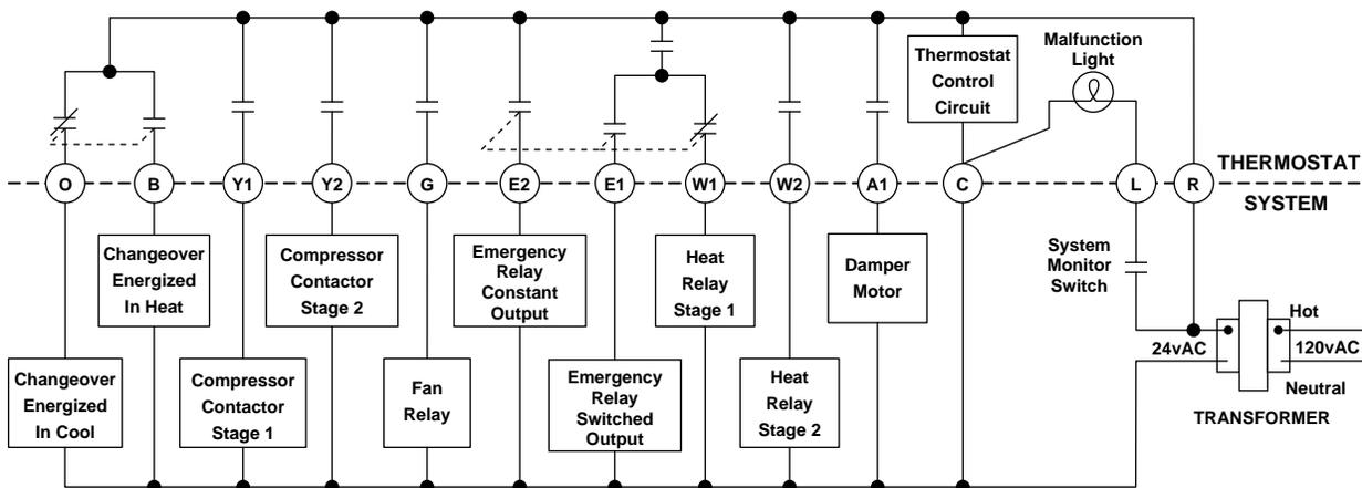
Figure 4. Typical wiring diagram for single transformer systems
