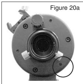
Figure 20a. Using the 2mm Allen wrench, turn the large screw counterclockwise a small amount, no more than 1/4 of a turn. (Note: Actual selected alignment screw will vary.)
