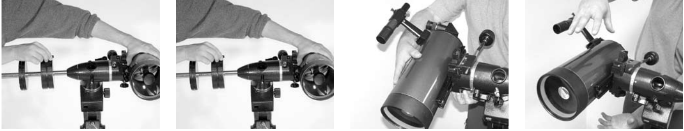
Figure 4a-d. Proper operation of the equatorial mount requires that the telescope tube be balanced on both the right ascension and Declination axes. (a) With the R.A. lock lever released, slide the counterweights along the counterweight shaft until it just counterbalances the tube. (b) When you let go with both hands, the tube should not drift up or down. (c) With the Dec. lock knob released, loosen the mounting plate securing knob and safety thumbscrew a few turns and slide the telescope forward or backward. (d) When the tube is balanced about the Dec. axis, it will not move when you let go.
