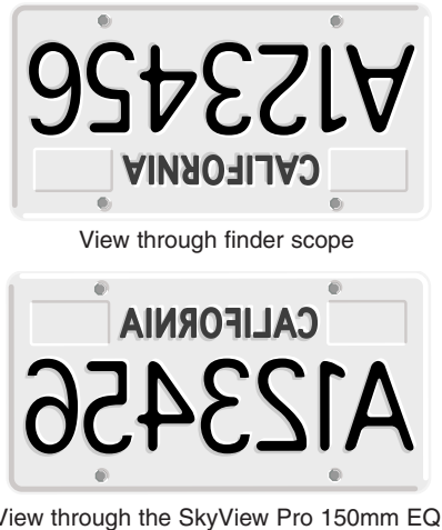
Figure 5. Images through the finder scope will appear upside-down and backwards (rotated 180°). Images through the SkyView Pro 150mm EQ with its diagonal in place will be reversed from left-to right.
