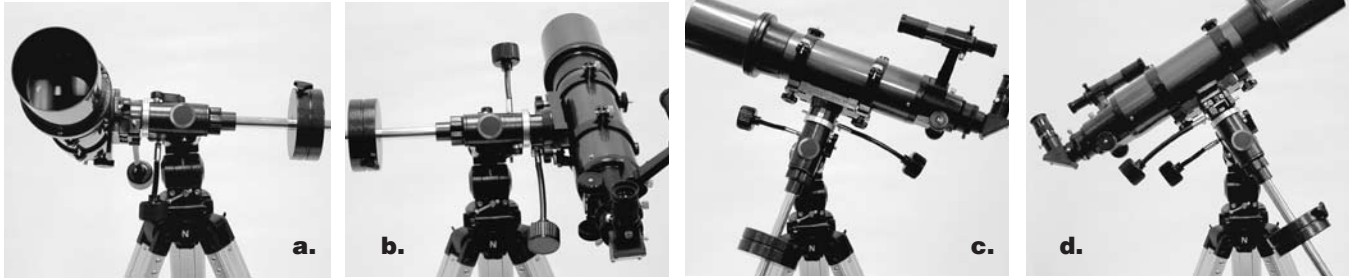
Figure 10 This illustration shows the telescope pointed in the four cardinal directions (a) North, (b) South, (c) East, (d) West. Note that the tripod and mount have not been moved; only the telescope tube has moved on the R.A. and Dec. axes
