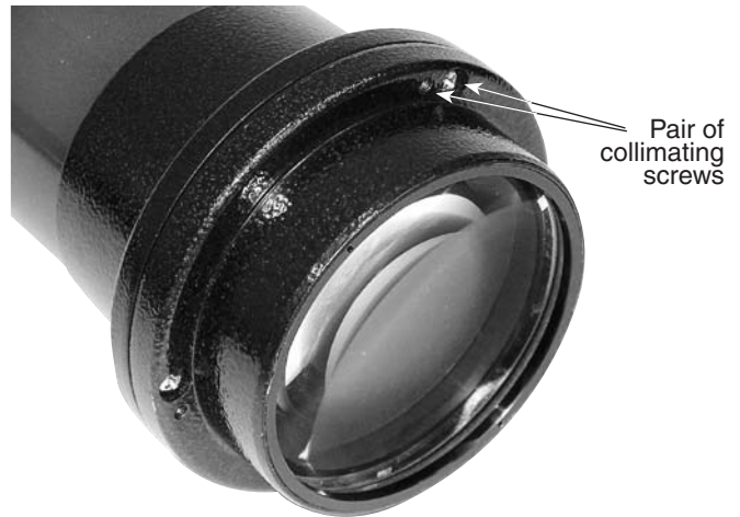
Figure 14. The lens cell of the AstroView 100. There are three pairs of collimating screws; each pair of screws work together to adjust the tilt of the lens.
