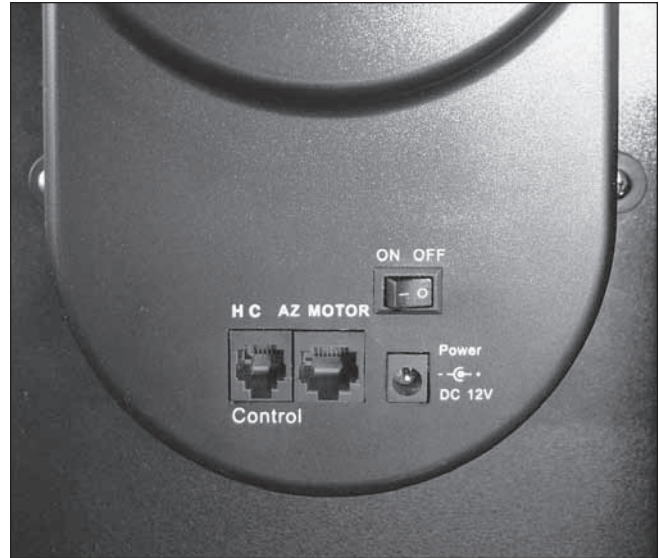
Figure 23. The altitude motor housing has the ON/OFF power switch and several cable ports.
