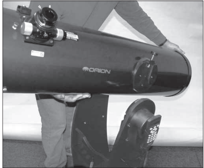
Figure 18. Hold the telescope tube as shown, with one hand on the rear end ring and the other cradling underneath the tube, gently lower the scope so the dovetail side bearing on the tube seats in the metal trunnion on the left side panel.
