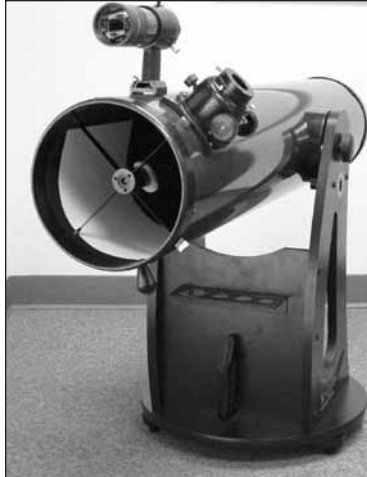
Figure 26. The SkyQuest optical tube properly set up for collimation. Note the white paper placed across from the focuser, and the level angle of the optical tube. Ideally, the telescope should be pointing at a white wall. (IntelliScope model shown.)
