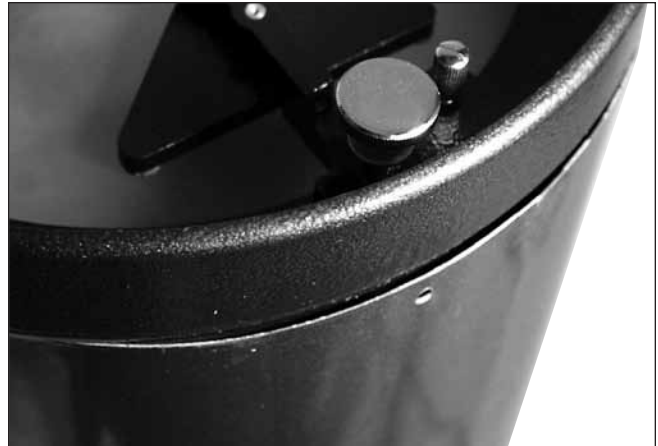
Figure 16. Locate the area of tube that is bulging out and preventing the end ring from fully seating.
