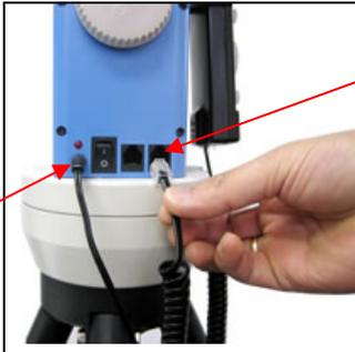
**Step 5. Plug in hand controller and AC adaptor.**
