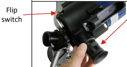
This picture shows the **eyepiece on the side**. Remove the protective cap to insert the eyepiece. The diagonal is not used for side viewing.
