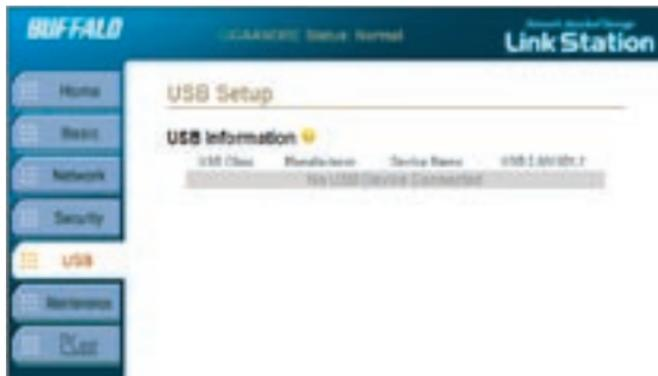
**USB Information:** The USB Information table lists information about connected USB devices (such as printers and hard drives). It lists the USB Class (Printer or Storage), the manufacturer if available, the device name, and whether it is a USB 1.1 or USB 2.0 device.
