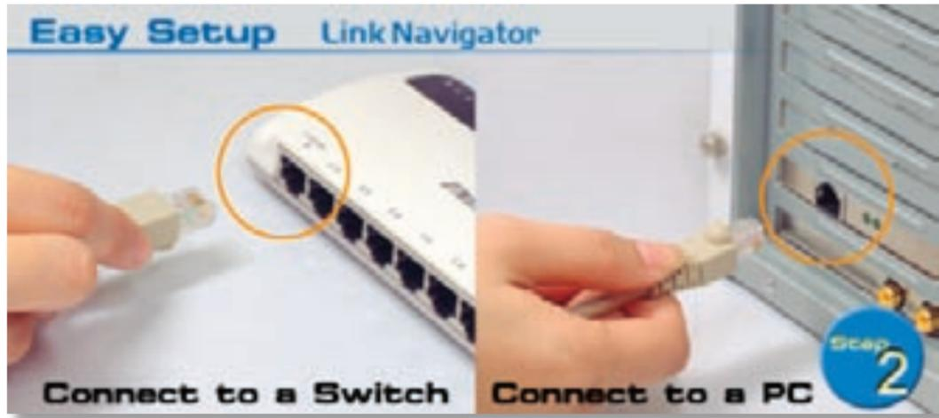
Connect the other end of the included Ethernet Cable into a hub, switch, or router on the network, or connect it directly to a nearby running PC.
