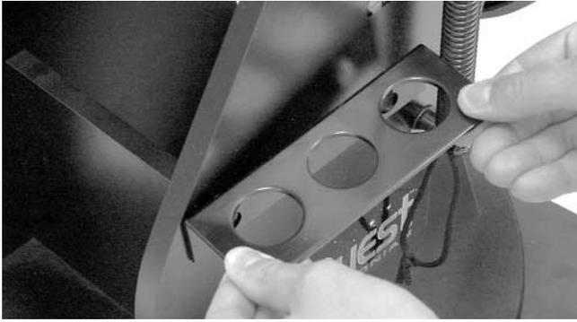
**Figure 4.** Using the two supplied screws, install the aluminum eyepiece rack in the predrilled holes about halfway down the left side panel of the base.
