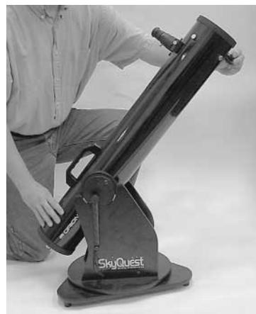
Figure 11: Try grasping the telescope as shown for easiest pointing. The left hand uses the Navigation Knob as a “handle”, while the right hand is on the rear of the tube.
