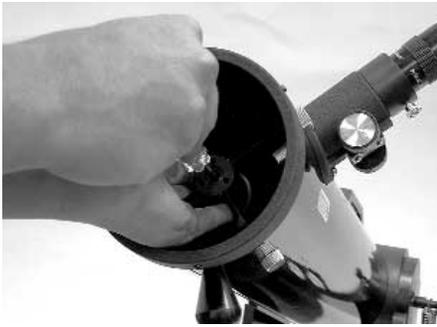
**Figure 17.** To center the secondary mirror under the focuser, hold the secondary mirror holder in place with your fingers while adjusting the center screw with the Phillips head screwdriver. Do not touch the mirror's surface.
