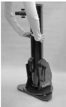
**Figure 5.** Set the optical tube on the "cradle" of the base so that the altitude side bearings on the tube rest on the white plastic "pads." Position the telescope as shown so that it won't fall down before the CorrecTension System is installed and engaged.
