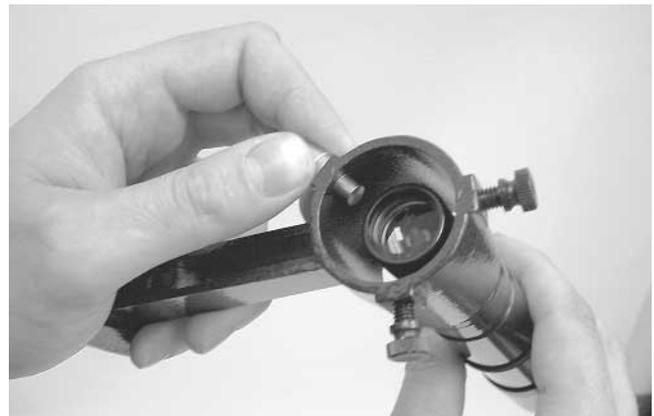
**Figure 8b:** Inserting the finder scope into the finder scope bracket
