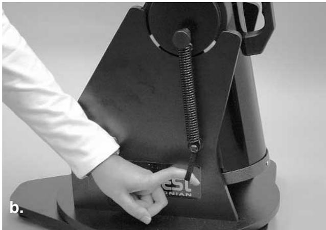
**Figure 7:** (a) To attach the spring to the base, grip the pull loop with your index finger and pull down on the spring. (b) While pulling down, slip the end ring of the spring over the screw head and onto the narrow part of the nylon spacer, then release the pull loop.
