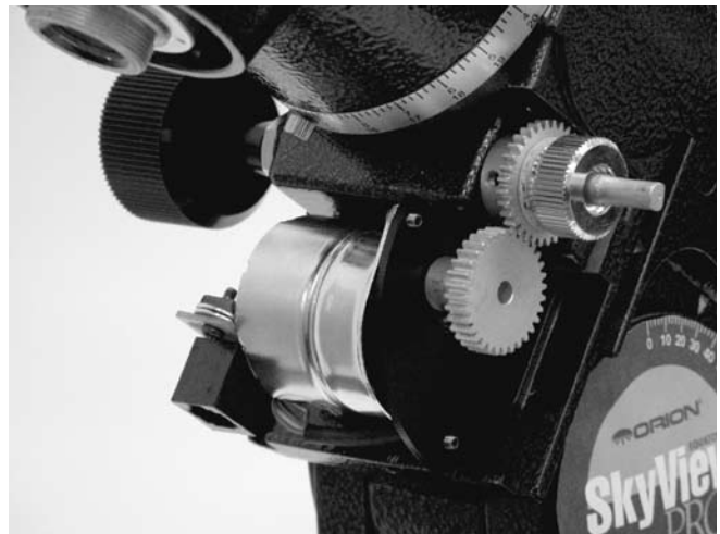
Figure 5. The assembled R.A. motor drive.
