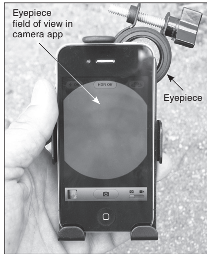
Figure 9. Position the telescope eyepiece so that its field of view is centered on the iPhone’s display.
