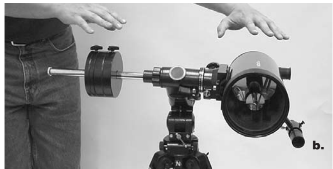
Figure 5a and 5b. Proper operation of the equatorial mount requires balancing the telescope tube on the R.A. axis. (a) With the R.A. lock knob released, slide the counterweight along the counterweight shaft until it just counterbalances the tube. (b) When you let go with both hands, the tube should not drift up or down.
