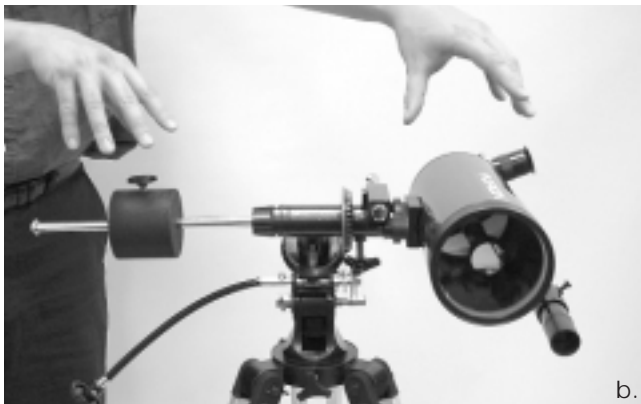
Figure 4a, b. Proper operation of the equatorial mount requires balancing the telescope tube on the R.A. axis. (a) With the R.A. lock knob released, slide the counterweight along the counterweight shaft until it just counterbalances the tube. (b) When you let go with both hands, the tube should not drift up or down.
