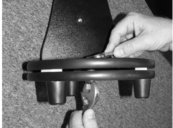
Figure 11: Making optional adjustments to the azimuth tension
