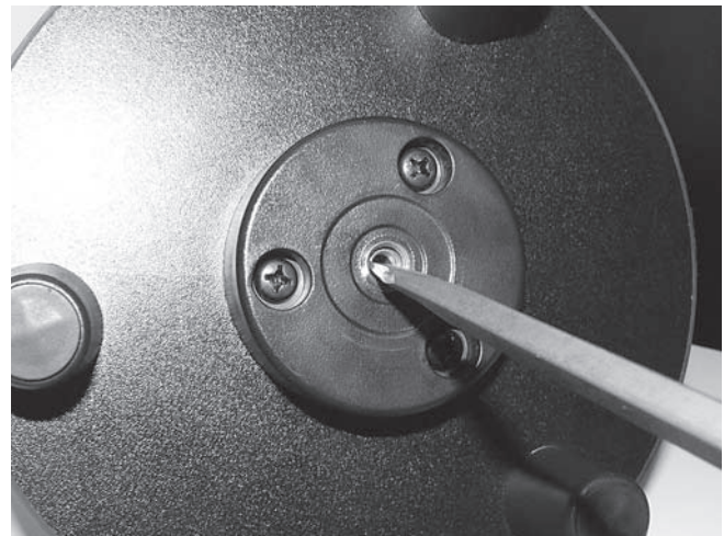
Figure 9b: Removing the 1/4"-20 adapter
