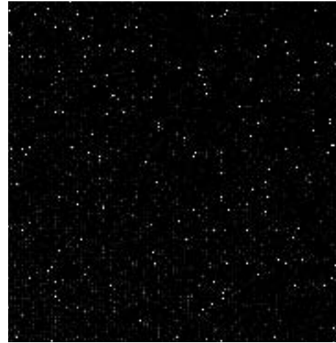
Figure 14. A dark frame contains the background noise. The same background noise appears in your "light" images. Dark frames isolate the noise so it can later be subtracted from your "light" images.
