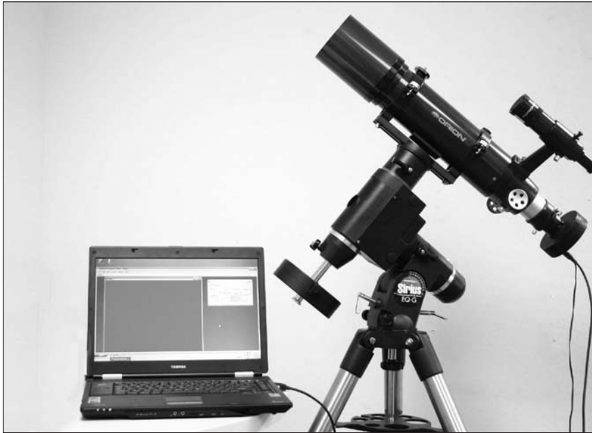
Figure 1. To use the StarShoot Pro, a telescope, mount, and computer are required. An autoguiding system is recommended.
