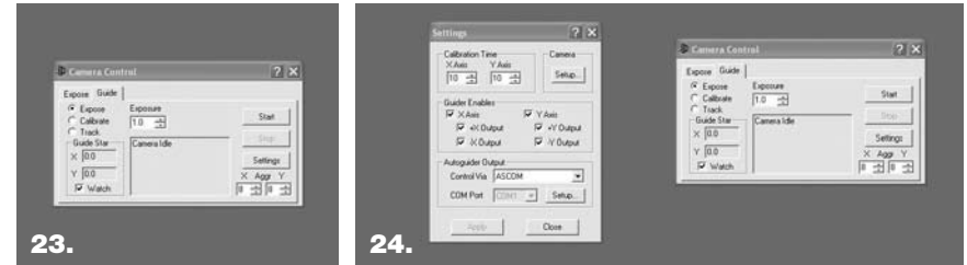
Figure 23. The Guide tab in the Camera Control Window is where the StarShoot Pro's autoguider functions can be accessed.
