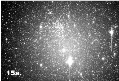
Figure 15a. Larger format CCD cameras like the StarShoot Pro reveal vignetting through most telescopes. Vignetting occurs when the edge of the image plane has less illumination than the center.
