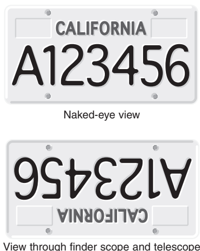
Figure 5. The view through a standard finder scope and reflector telescope is upside down (rotated 180°). This is true for the SpaceProbe 130mm and its finder scope as well.
