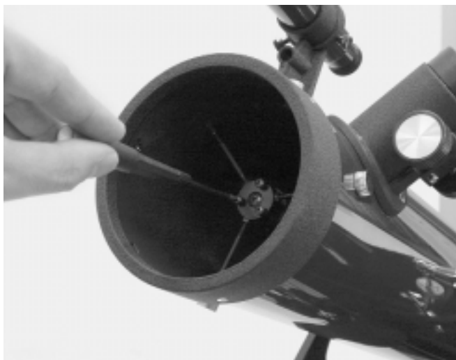
Figure 8. Adjust the tilt of the secondary mirror by loosening or tightening the three alignment screws with a small Phillips head screwdriver.
