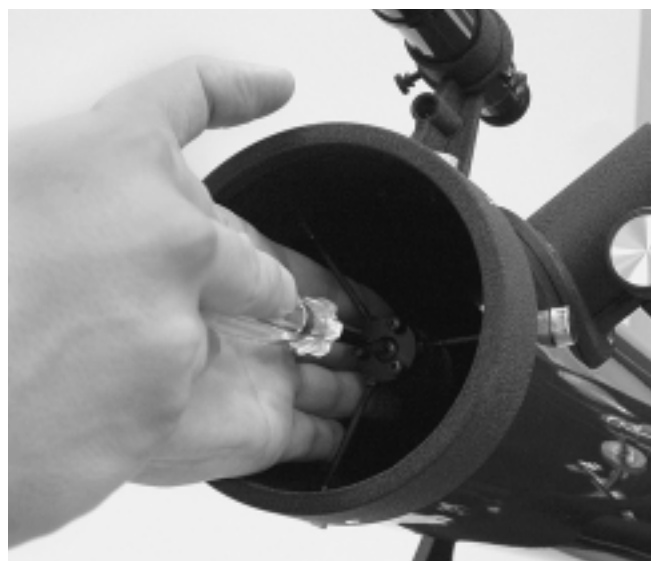
Figure 7. To center the secondary mirror under the focuser, hold the secondary in place with your fingers while adjusting the primary screw with a Phillips head screwdriver. Do not touch the mirror's surface.
