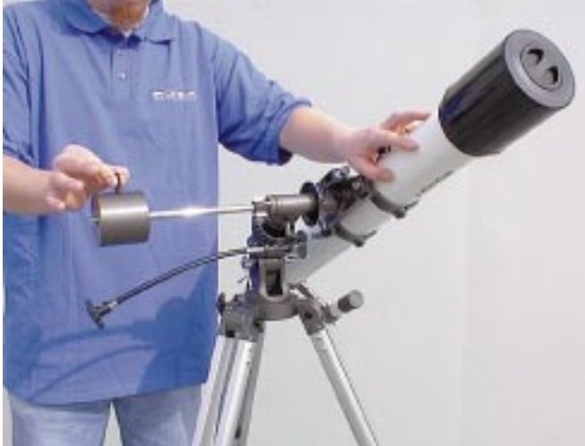
Figure 2a. Balancing the telescope with respect to the R.A. axis by sliding the counterweight along its shaft.
