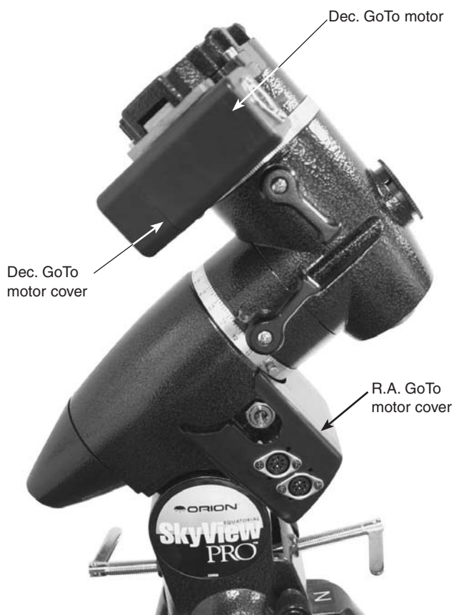
Figure 12. Installed GoTo motors
