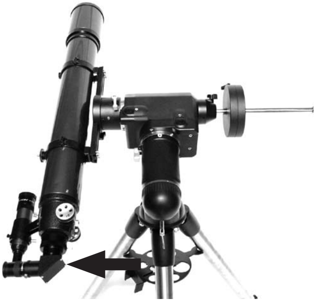
Figure 20. gently push the telescope horizontally to determine direction of optical axis offset.
